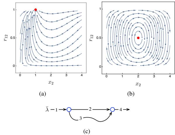
Fig. 4. Dynamical behavior of two parallel highways (schematized in (c)). Travel costs are as follows:  $\tau_2(x_2) = x_2$  and  $\tau_3(x_3) = \bar{\tau}_3 = 2$ . (a) Phase portrait for non-saturated freeway:  $\bar{\lambda} = 0.5$ ,  $v_2 = 0.5$ , (b) Phase portrait for saturated freeway:  $\bar{\lambda} = 1$ ,  $C_2 = 1$ . Red dots show equilibrium points.
