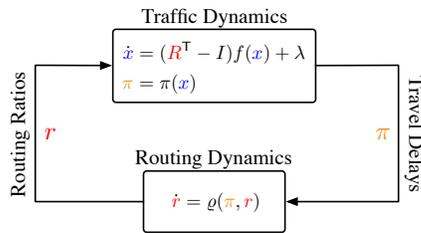
Fig. 3. Feedback interconnection between traffic and routing dynamics.
