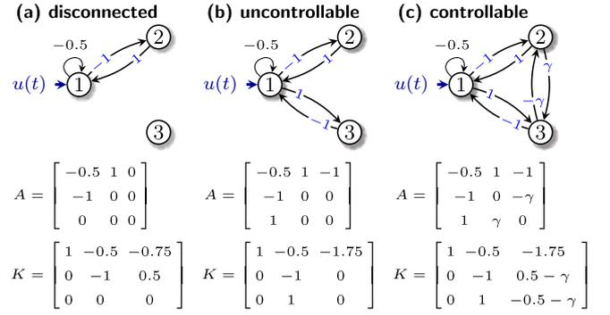
**Fig. 2.** The three networks are all diagonally admissible for  $W = \text{diag}(1, 1, 1)$  because they satisfy  $A + A^T = -BB^T$  where  $B = [1, 0, 0]^T$ . Network (a) is disconnected and uncontrollable. Network (b) is connected but uncontrollable. Network (c) is controllable.
