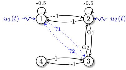
**Fig. 3.** Given  $W = \text{diag}(1, 1, 1, 1)$  and  $B = [e_1, e_2]$ , the chain network, which contains one single spanning path  $(1, 2, 3, 4)$ , is controllable and diagonally admissible for  $W$  when  $\alpha_1/\alpha_2 = -1$ . The network remains controllable and diagonally admissible for  $W$  when the dotted edges are added with  $\gamma_1/\gamma_2 = -1$ .
