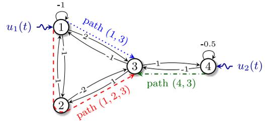
$$A = \begin{bmatrix} -1 & 1 & -1 & 0 \\ -1 & 0 & 1 & 0 \\ 2 & -2 & 0 & -1 \\ 0 & 0 & 1 & -0.5 \end{bmatrix}, \quad B = \begin{bmatrix} 1 & 0 \\ 0 & 0 \\ 0 & 0 \\ 0 & 1 \end{bmatrix}, \quad W = \begin{bmatrix} 0.5 & 0 & 0 & 0 \\ 0 & 0.5 & 0 & 0 \\ 0 & 0 & 1 & 0 \\ 0 & 0 & 0 & 1 \end{bmatrix}$$
